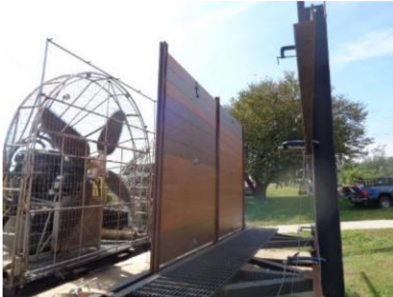
Photo No. 1 Test Specimen in Rigid Test Fixture with Transducers
