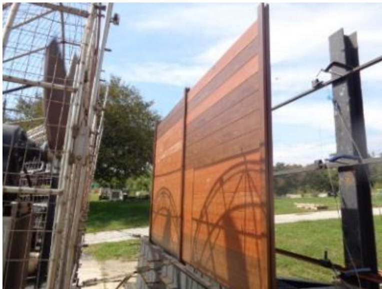
Photo No. 2 Wind Generator Outlet Relative to Test Specimen
